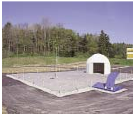
Open area test site for calibration and measurement at 10 and 30 m
