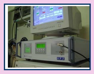
The CL55C main characteristic, is its ability to sample, in parallel, the peak and quasipeak levels of the four channels, to recognize and count all clicks (short, long, continuous noise and switching operations), and store all numeric and graphic data, like waveforms, in the PC hard disk.
