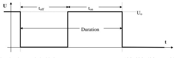
Load resistor, switch able  $R_s$ Switch-off time,  $t_{off}$ , adjustable Switch-on time,  $t_{on}$ , adjustable Number of Pulses, adjustable 10Ω, 20Ω, 40Ω, ext. >2Ω 1 ... 1000s 1 ... 1000ms
