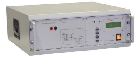
The Electronic Power Switch EPS 25 can be used for simulation of fast supply voltage dropouts as required by various vehicle manufacturer standards, e.g. PSA 217110 (micro-cut-off with real interruption); see table below.
